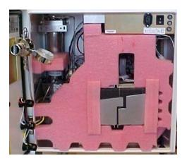
Figure 11: Internal Foam Support
